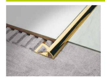
The ROUNDTEC RD profile is mainly used in transitioning floor types of different thicknesses, for example from ceramic tile to thin linoleum. Its rounded section provides a smooth level change of 1/8" (3mm), making it suitable between two floor types or as an end profile. ROUNDTEC can even be used as stair nosing or edging for tile countertops. Available in brass with patented dovetail anchoring.
